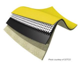
A unique waterproofing membrane composite with a 60-ml-thick thermoplastic membrane reinforced with a weft polyester knit fabric and a hydrophilic polymer layer that will activate and swell at any breach in the thermoplastic membrane to stop water ingress.
