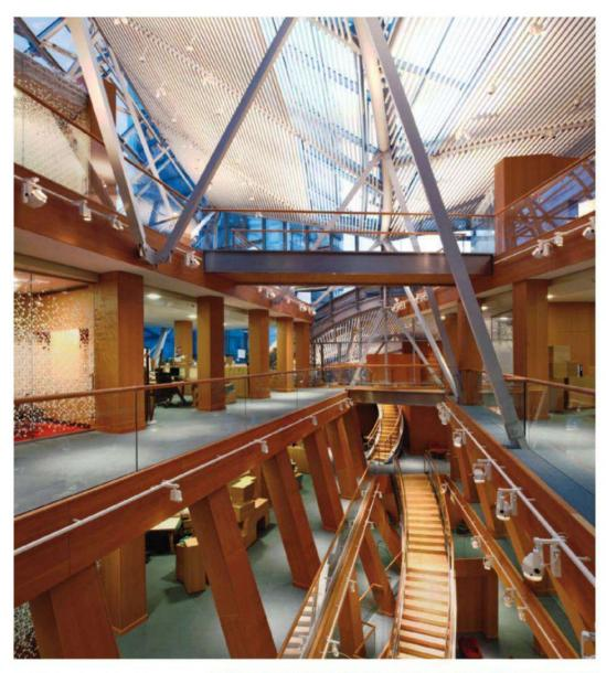
ABOVE: A central atrium brings daylight to interior Gehry-designed workstations and glass-enclosed "private rooms" at the heart of the office floors. Adjustable metal-halide up and downlights illuminate this space when necessary and reflect off overhead white lamellas (a radiator-like array that also diffuses sunlight from the glass roof and provides radiant cooling).
