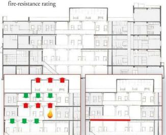
**Top:** Cross-sectional view of office showing offset configuration of floor openings; **Bottom left:** Smoke exhaust control system design; **Bottom right:** Horizontal flexible smoke curtain at second floor
