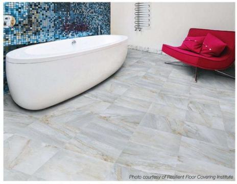
Within Standard 332, resilient flooring is specifically defined as "a floor surfacing material made in sheet or tile form, or formed in place as a seamless material that has a wearing surface that is not textile." The resilient flooring above has the appearance of stone, but is not.
