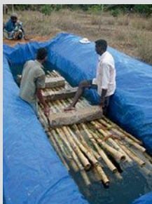
Bamboo treatment – Dip diffusion
