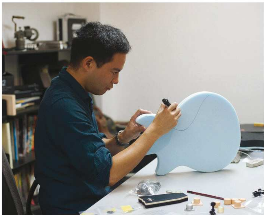
ABOVE Creating 3D models of the guitar enabled the designers to get a real feel of the instruments and add in, as pictured, the ideas for the body contours. Here’s chief designer, Toshihide Suzuki at work
