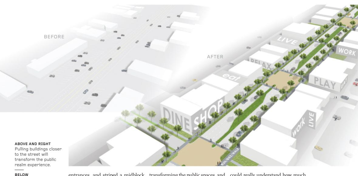
The illustrative site plan shows proposed improvements in lane configurations, medians, and intersections.
