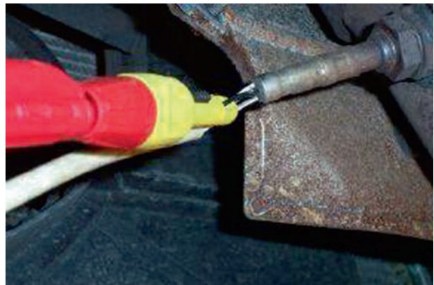
Figure 4.23 Titania knock sensor in position
