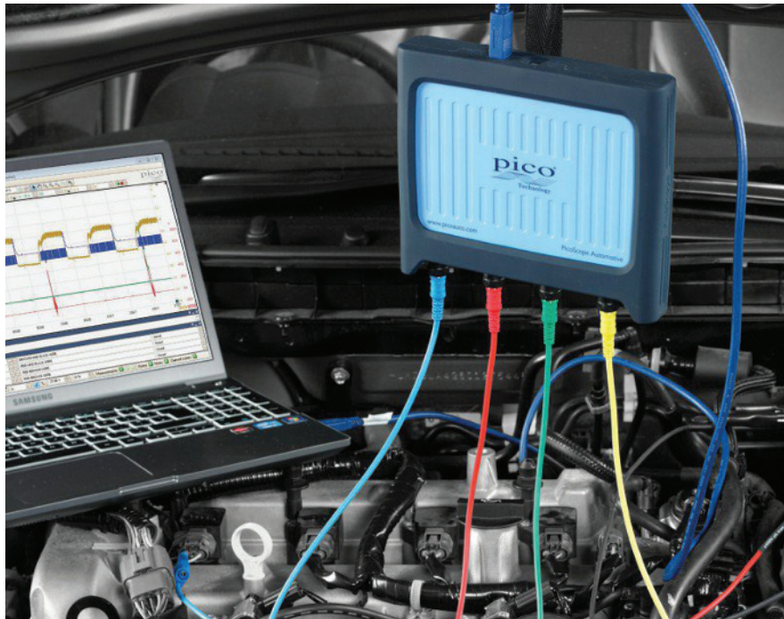
Figure 3.7 A PicoScope and laptop with connections to engine components (Source: PicoScope)
