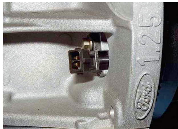
Figure 4.1 Crank sensor in position near the engine flywheel
