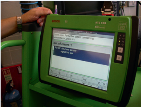
Figure 3.32 Take a readout from the control unit memory (DTC display)
