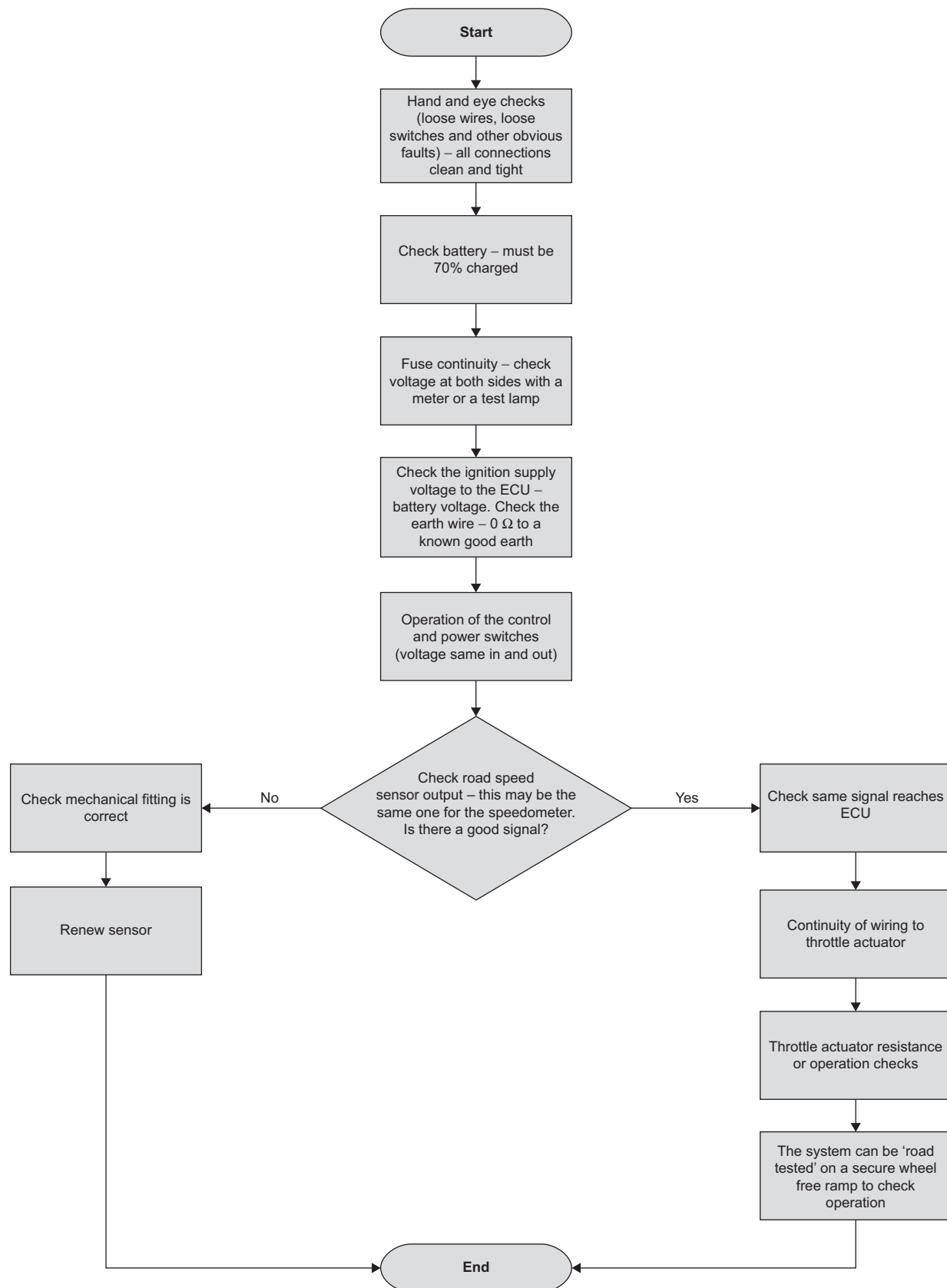
Figure 8.83 Cruise control fault diagnosis chart
