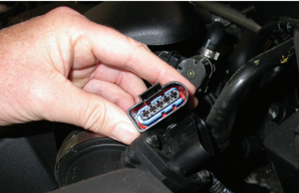
Figure 6.68 Airflow meter under test
