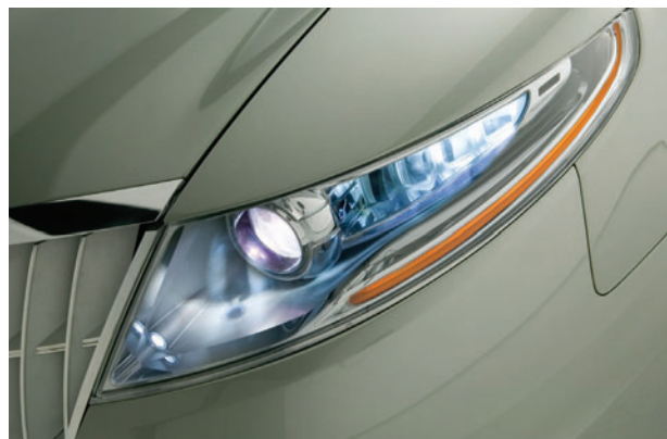
Figure 8.27 Adaptive lighting using LEDs
