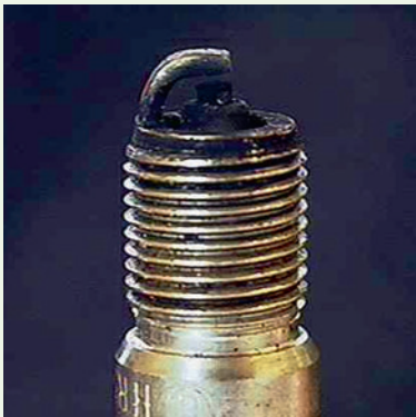
Figure 6.32 Carbon fouled (standard plug)
