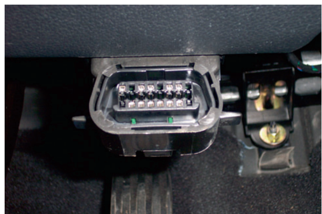
Figure 4.68 DLC socket – pin 6 is CAN high and pin 14 is CAN low
