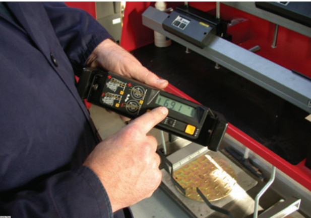
Figure 7.26 Laser alignment systems give digital readouts
