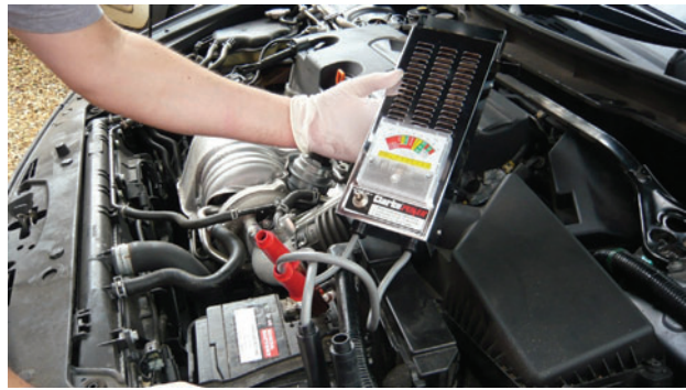
Figure 6.90 A high-rate discharge tester can indicate battery state-of-health, but still relies on the skill and judgement of the technician. In addition, there are several health and safety-related issues to this approach! Note the tester in the picture is a fixed load, and not really suitable for the battery shown (Source: www.autoelelex.co.uk )
