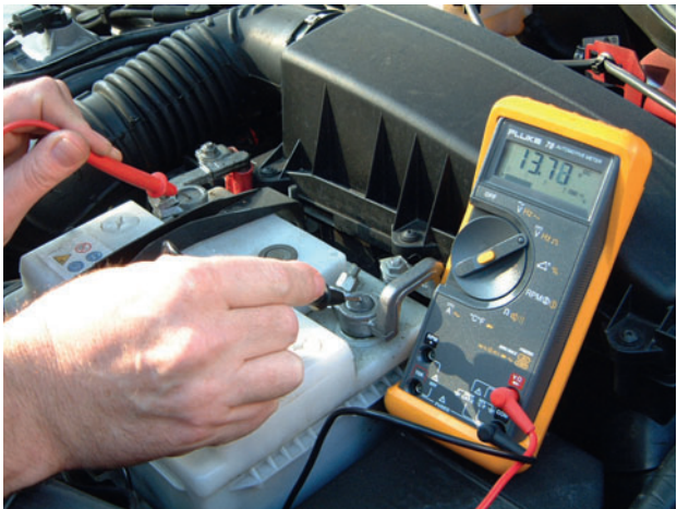
Figure 6.88 Checking battery voltage. In this case, the engine had just been switched off so the reading shows a ‘surface charge’
