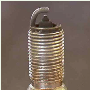
Figure 6.35 Carbon fouled (platinum plug)
