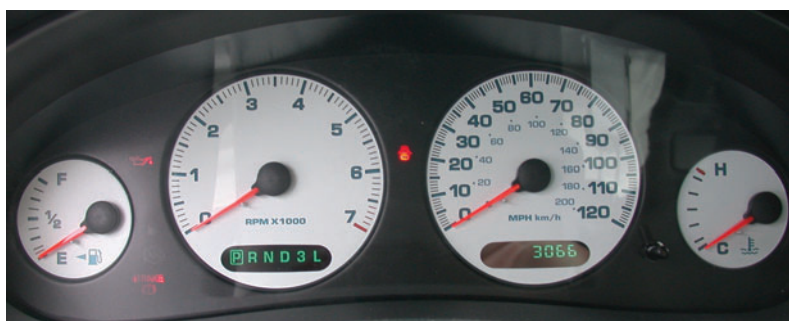
Figure 8.68 Instrument display combining analogue and digital displays
