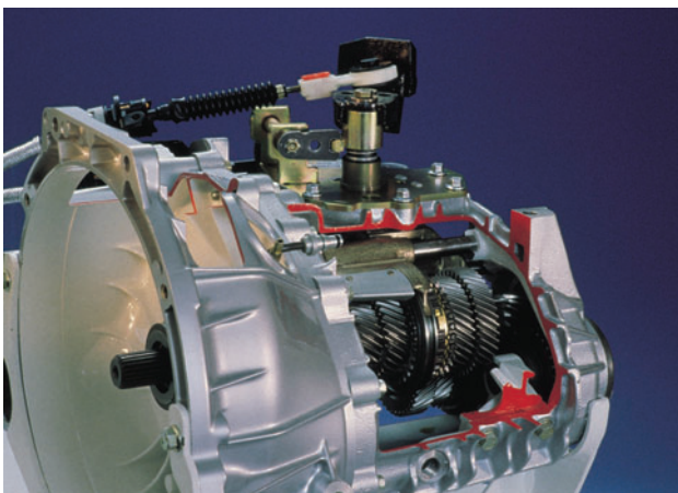
Figure 9.3 Manual gearbox with a cable change mechanism (Source: Ford Media)
