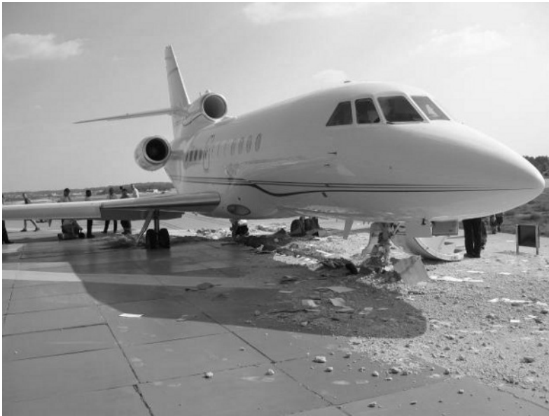
Figure 5-4 The Dassault Falcon 900 business jet successfully arrested by the ZODIAC-ESCO EMAS system at Greenville Downtown airport on 17 Jul 2006 (Courtesy ESCO ZODIAC, photo: David J. Heald, C.M.)
