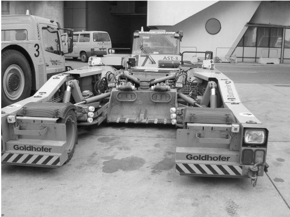
Figure 9-8 Heavy Goldhofer towbarless tractor (Photo: A. Kazda)
