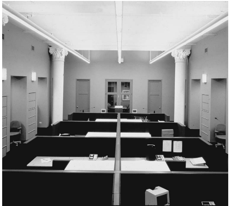
Figure 3.10 An example of diffuse upward distribution.
