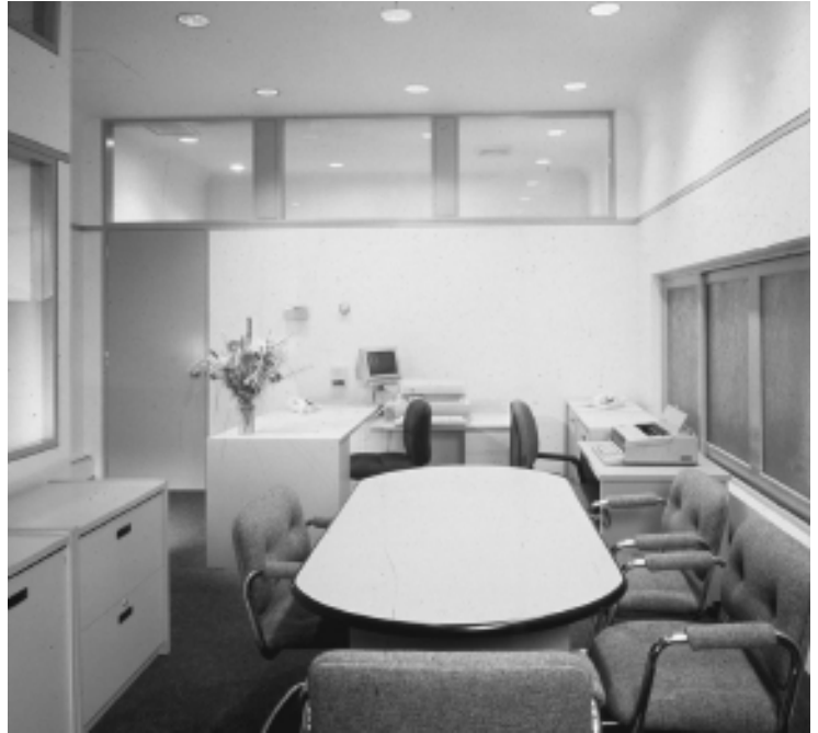
Figure 3.5 An example of diffuse downward distribution.
