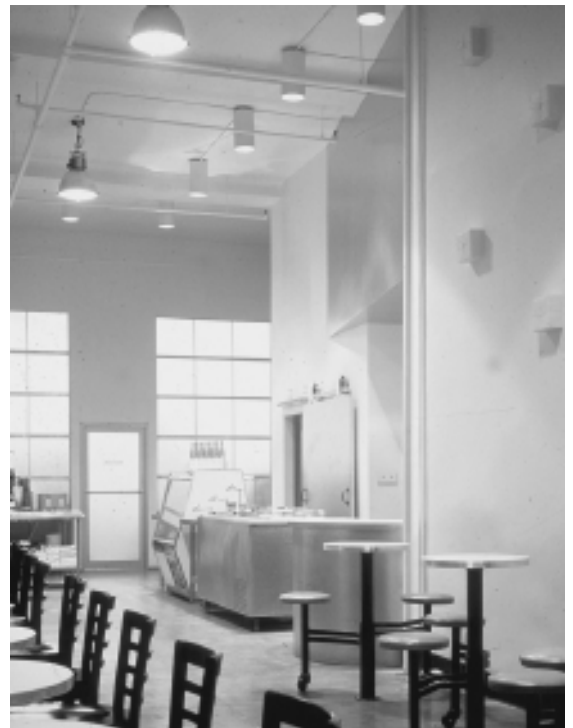
Figures 3.19 and 3.20 If all of the room surfaces are light-colored, interreflections will fill in shadows and reduce contrast.
