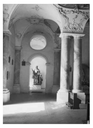
Figure 3.5 Zwiefalten Abbey in Bavaria, where the structure of the nave is designed as giant vertical louvres to modify the daylight entering the building. (Copyright James Bell)
