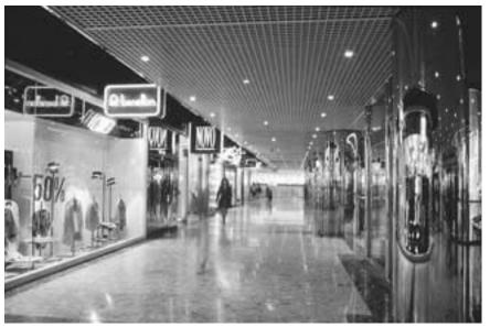
Figure 3.9 An underground shopping arcade at Sha Tin in Hong Kong where the lighting is changed from day to night. During the day (see Figure 3.8) fluorescent lighting is used whilst at night filament sources are employed (see Figure 3.9), both above a louvred ceiling. (Photographer Derek Phillips)
