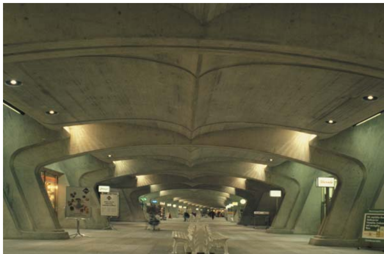
▲ 7.51 Stadelhofen Railway Station, Zürich, Switzerland, Santiago Calatrava, 1990. Cambering the beams and the 'sloping columns' visually lighten the shopping mall.
